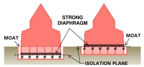
Figure 5. Key requirements of a base isolation scheme
