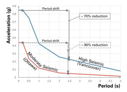
Figure 6. Seismic force reduction due to fundamental period shift caused by base isolation
