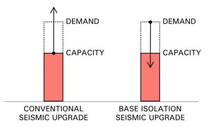
Figure 4. Conceptual difference between a conventional vs. base isolation seismic upgrade approach
